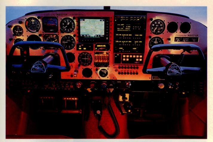
This pristine Comanche 250 is a blend of old and new. Original instruments merge with a full UPS Aviation Technologies stack, a Century 2000 autopilot, and much more. The trademark Piper control yoke of the 1950s to 1970s—the "square pretzel"—features the Comanche logo, a streamlined bird cruising among the stars.
